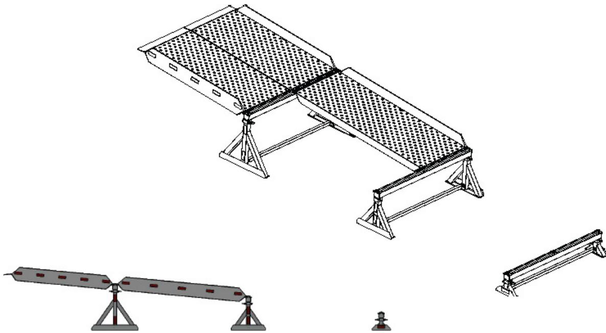
**Step 4.** With both upper ramps installed, and the upper middle ramps installed, repeat with the lower middle ramps. Check the position of the lowest stand. Adjust as needed. Install the last middle ramp. (All four middle ramps are the same.)
