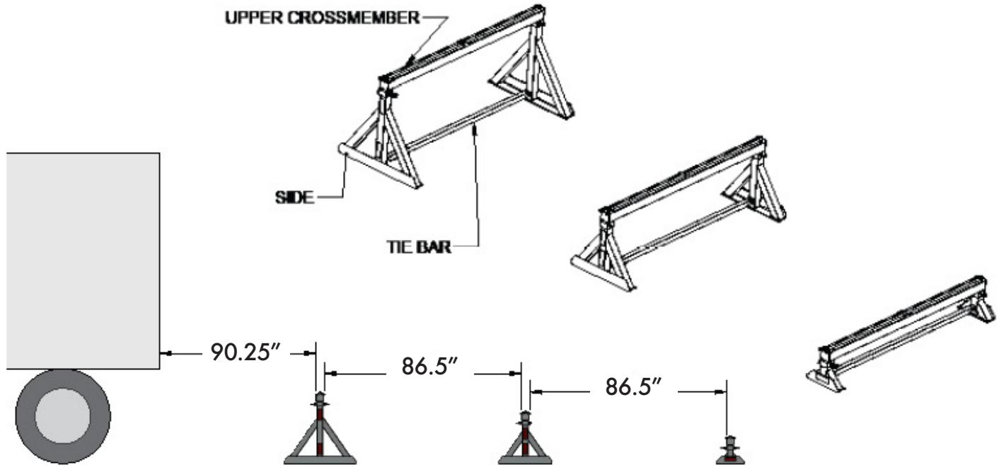
**Step 2.** Install one of the upper ramps making sure the tallest stand is in position to the trailer/dock. Reposition the stands as necessary. Install the other upper ramp.
