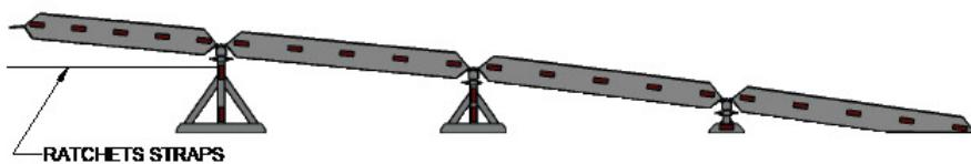
**Step 6.** Install the two ratchet safety straps, attaching them from the upper stand to the ICC bumper.
