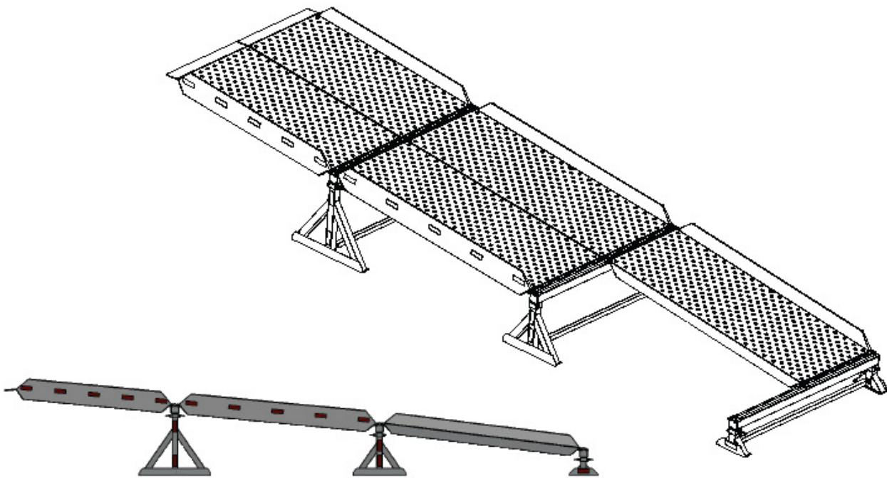
**Step 5.** Install the lower ramps. With all the ramps in place, install the steel rods to secure the ramps to the stands. Make sure each rod is secured with an R-clip.
