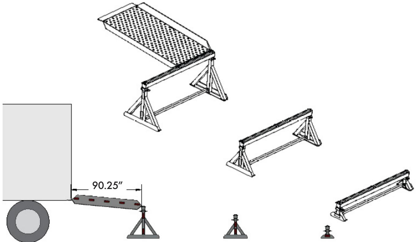
**Step 3.** Install one of the upper ramps making sure the tallest stand is in position to the trailer/dock. Reposition the stands as necessary. Install the other upper ramp.
