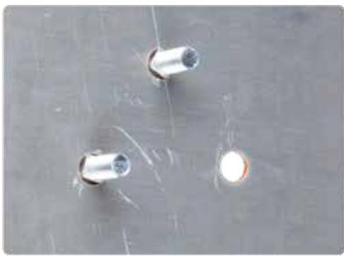
**Step 2.** Align the bolts in the dock plate with the holes of the stabilizer. Push through until the base of the stabilizer is against the dock plate.
