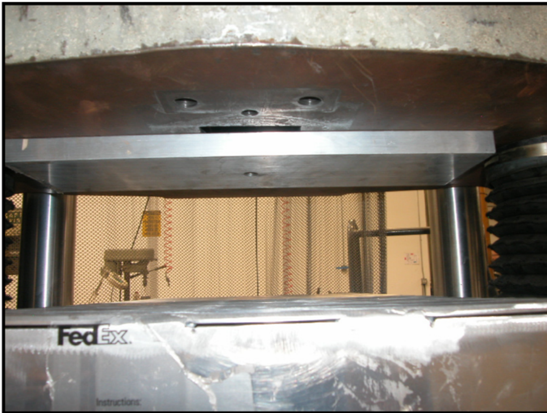
Photograph 4: Compression test setup: Compressive aluminum plate
