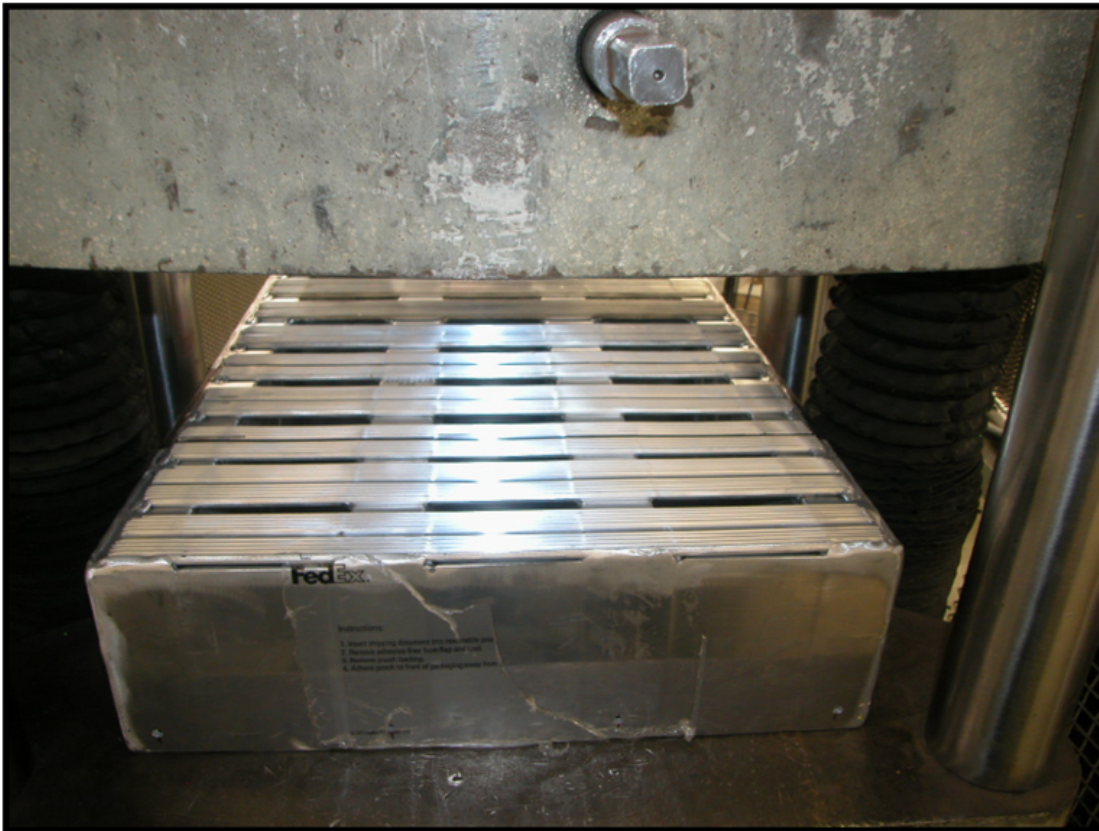
Photograph 2: Compression test setup: Bus platform under the 400kip frame
