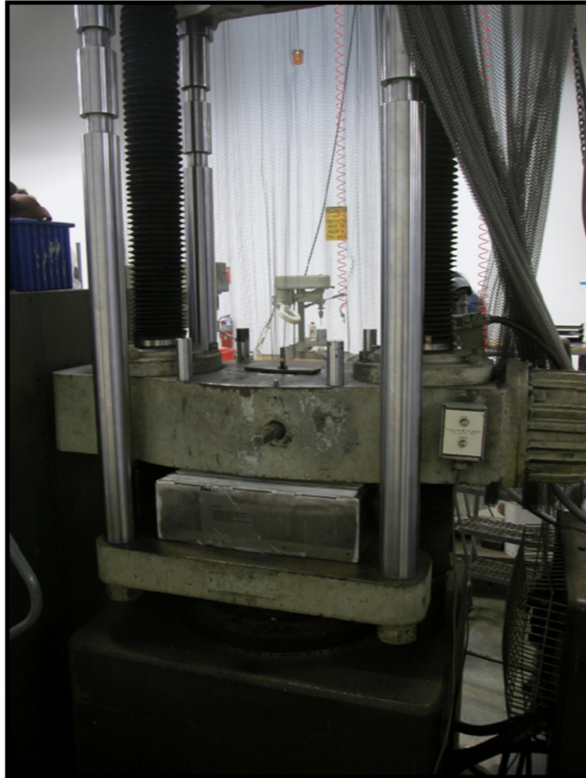
Photograph 1: Compression test setup: Bus platform in test position
